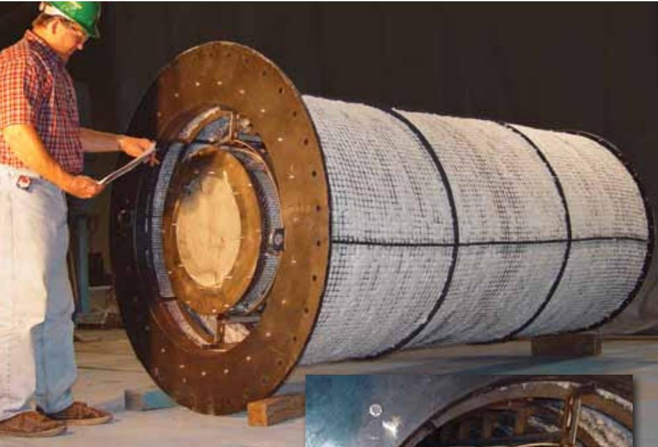
A new Brink® Pt Filter in a concentric design, features an internal cage type structure and robust construction.
