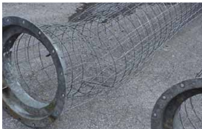
Before repair and repack – mishandling of this fiberbed has caused serious damage to the cage and flange of this stripped element.
