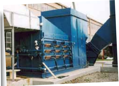
Prefiler and heat exchanger module
