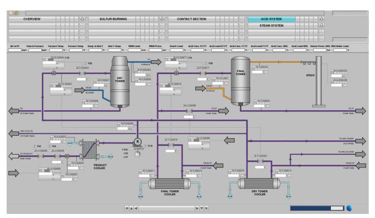
Elessent operator training simulators can be fully customized, allowing you to create a training environment that is as close to your real unit as possible; customization may include tag names, DCS screens, process configuration, control logic and equipment sizes.
